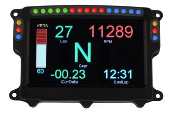
The PCU-8D is a lightweight driver display module designed for general motorsport applications. It is designed to connect to a host ECU via CAN and present the driver with information on a 4.3" display and LED lamps. The display is suitable for use in direct sunlight and at night. The text and graphics layout of the screen is user-configurable via PC software. 100 pages are available, and are selectable by CAN message.
